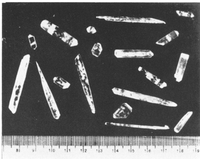
Figure 2 A photograph of some of the crystals grown in gels.
